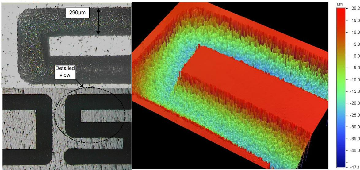
Fig 11. Microchannels: optical and profilometer 3D image.
