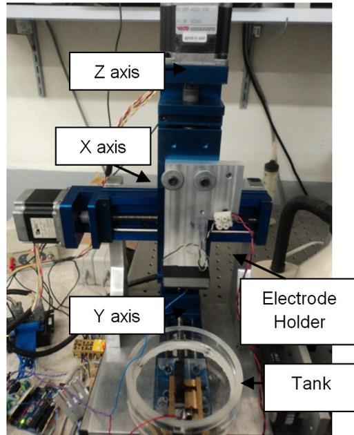
Fig 12. Gantry configuration for control system portability test.
