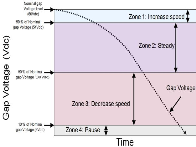
Fig 8. Gap voltage zones specified for gap control.
