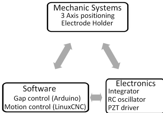
Fig 1. Micro EDM machine architecture and subsystems.
