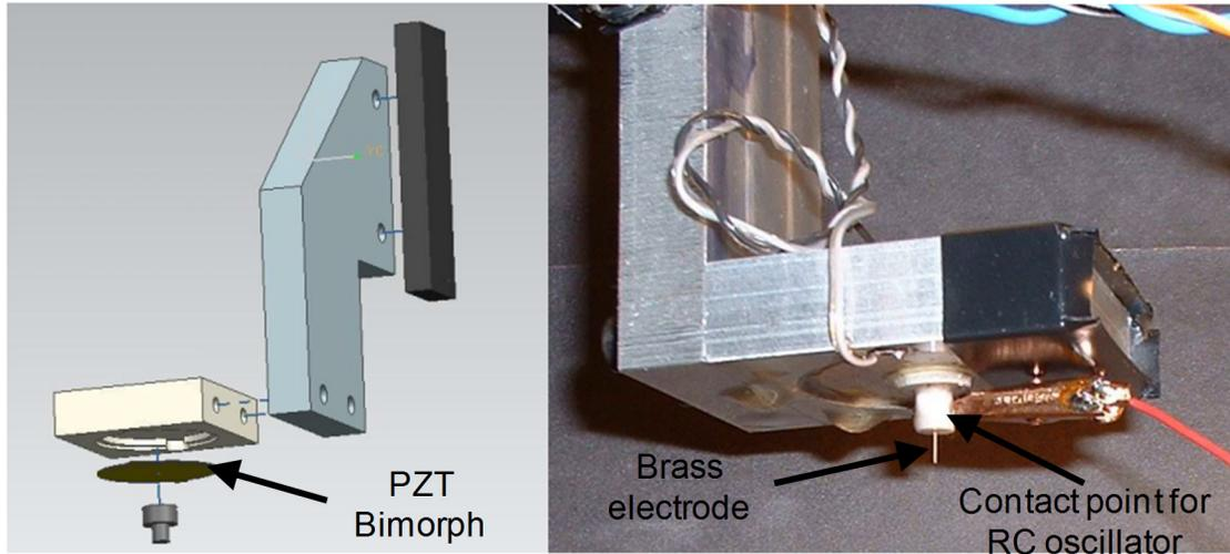
Fig 5. Electrode holder, a) CAD model. b) Assembly.
