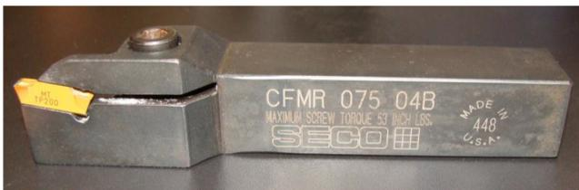
**Figure 2.** Cutting tool holder and grooving insert.
