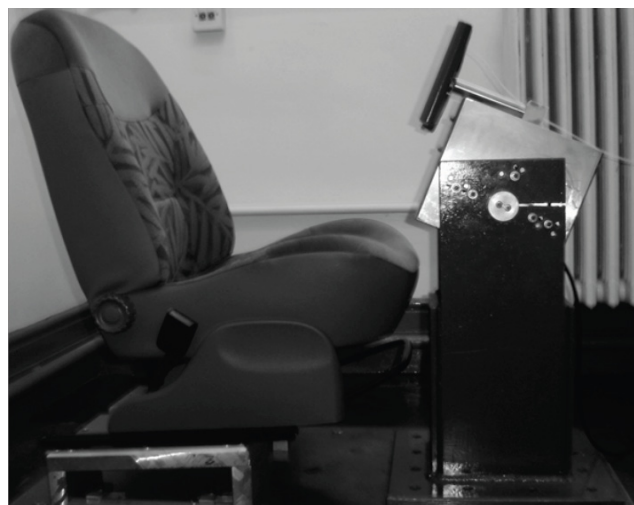
Figure 6: Steering wheel vertical vibration test facility.
