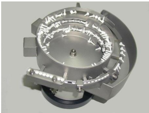
Fig.25. Vibratory feeder with orientation of elements
