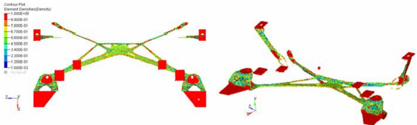
Figure 8 Subframe structure after the optimization process.
