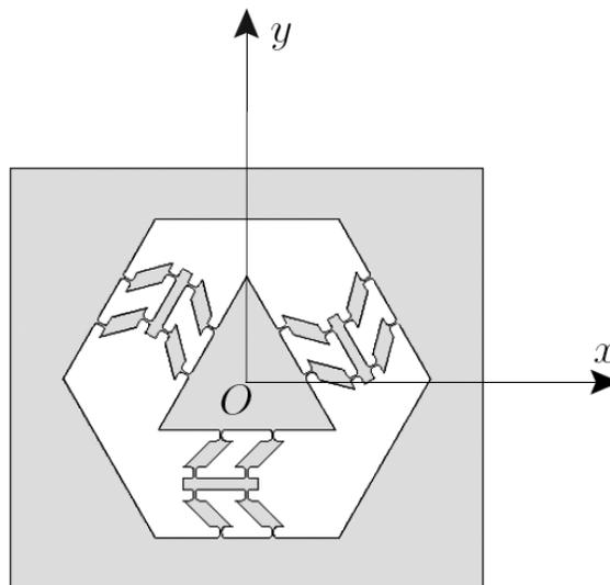
Figure 1: A biaxial accelerometer with simplicial architecture
