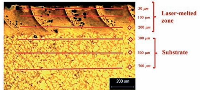
Figure 7 – OM image in the cross section of Al-Fe sample laser-treated, indicating the depths selected for microhardness measurements.
