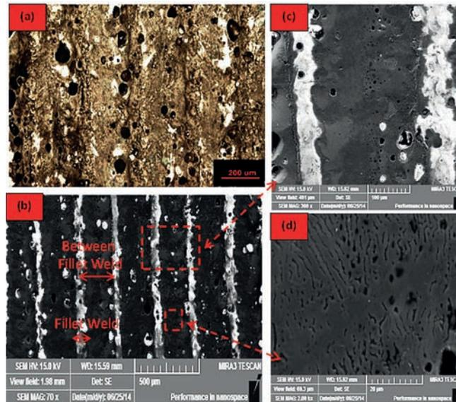
**Figure 2** – (a) OM, and (b) FESEM images of the morphology of hypereutectic Al-2.0 wt% Fe alloy LSR-treated surface, showing regions on the weld fillet and between the weld fillets, (c) on the weld fillet region at increase magnification, and (d) between weld fillets region under higher magnification.
