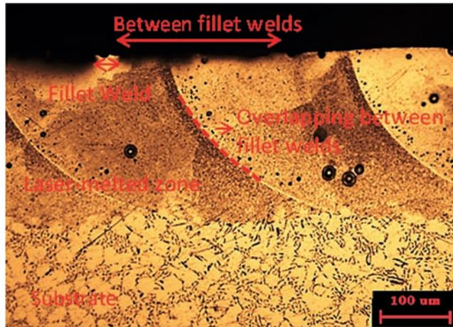
Figure 3 – OM micrograph in the cross sectional area of laser-treated material
