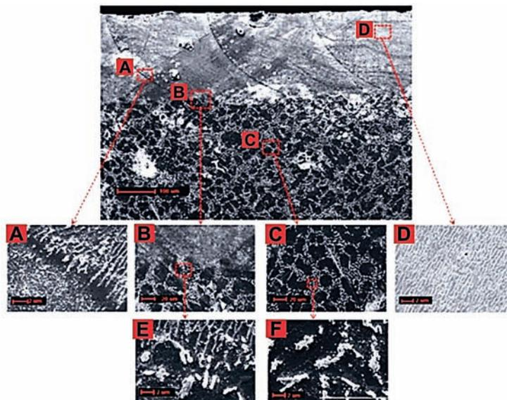
Figure 4 – SEM micrograph in the cross-sectional sample of Al-2.0 wt.% Fe alloy LSR-treated: (a) overlapping line of consecutive weld fillets, (b) interface of treated surface and substrate, (c) substrate unaffected by laser treatment, (d) detail in the cast region. (e) interfacial region of the treated surface and substrate, and (f) detail of the substrate unaffected by laser treatment.
