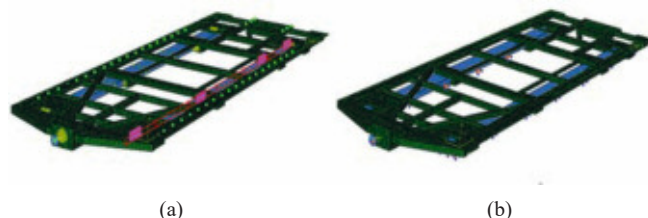
Figure 11. Finite element model with rails, (a) Tangent contact and (b) Spatial constraints.
