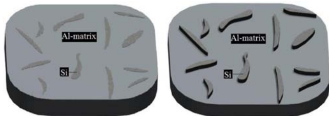
Figure 4. Schematic representation of the exposure of silicon particles as a consequence of Al-matrix removal during the wear test.
